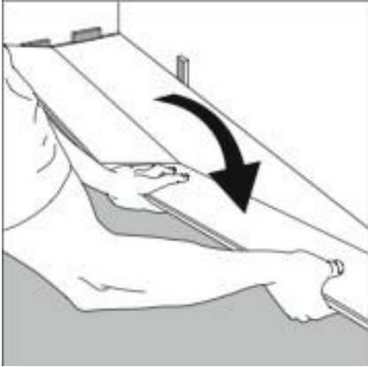
Fig 7. Second plank second row. Place the short end of the floorboard at an angle against the previous installed floorboard and fold down all the way.
