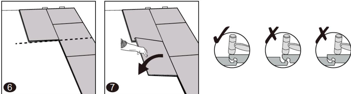
8. After finishing the installation of each row: Use scrap pieces and a small hammer or rubber mallet to gently tap the tiles into the click of the previous row to make sure they are tightly engaged together and make sure there is no gap between the long side of the tiles installed. Any gapping can compromise the whole installation.
