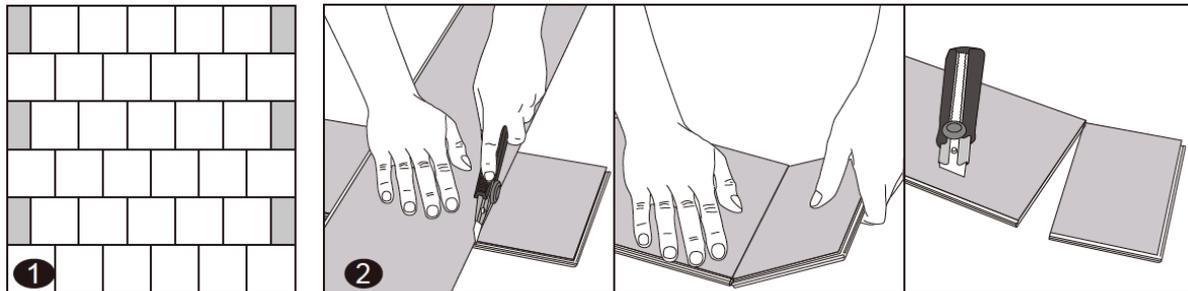
3. First row, first tile: After adjusting the measurements of the first panel as described above, begin laying at the left-hand corner of the longest wall and proceed from the wall with the tongue sides facing the wall and the groove facing outward (groove sides are marked with arrows on the back of each tile), away from the wall. Use spacers to create an 8mm expansion gap around the room.
